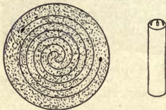
FIGURE 236.—DIAGRAM OF A DRY LEAD STORAGE BATTERY.
